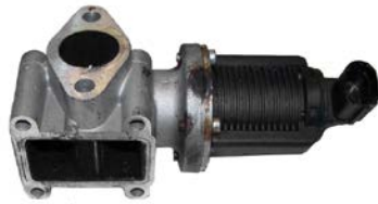
EGR valve (V40-63-0014) with soot deposits
