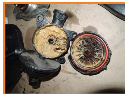
Residues in the oil trap, BMW 3(E90), X3
