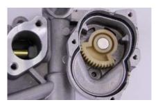
The magnetic field sensor allows a contactless determination of the position.
