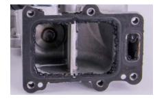
Pieces of the broken sealant can damage the thermostat and the water pump. Blockages may decrease the cooling efficiency.
